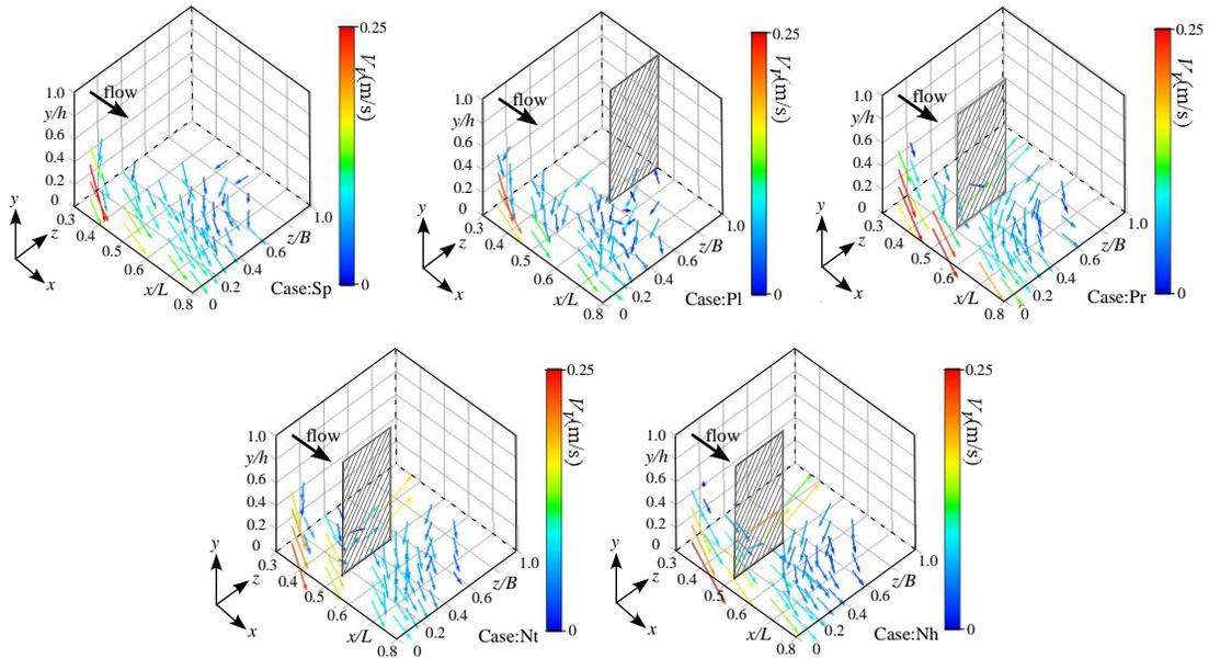
Fig. 7 Vector of flow velocity at nearly partition
