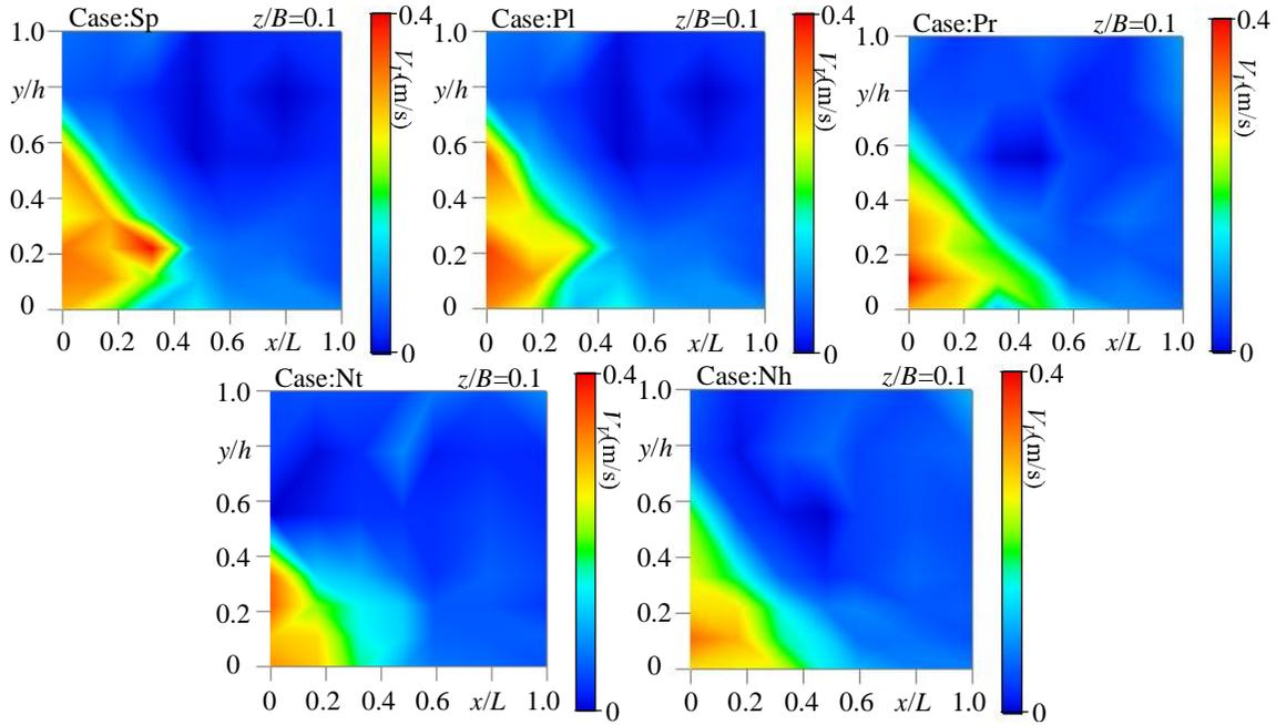
Fig. 6 Contour of flow velocity at  $z/B=0.1$  in vertical section
