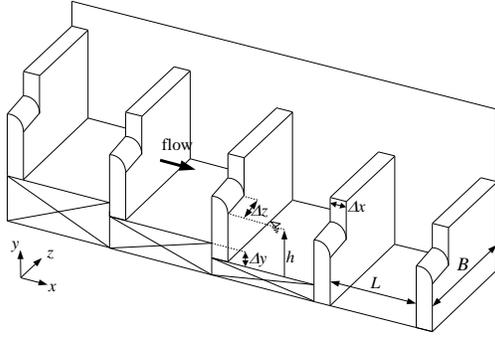
Fig. 1 Pool-and-weir fishway
